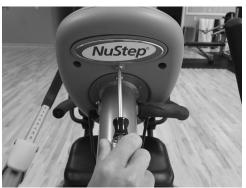
2. Replace the 4 AA alkaline batteries. (NiMH rechargeble batteries may also be used.)
